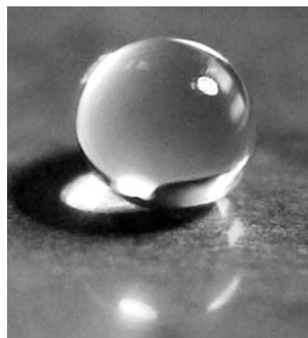
Figure 3. Water drop on the surface of the ultrahydrophobic multilayer surface from Figure 2. The diameter of the drop is about 2 mm.
